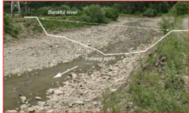
Fig. 2. Dimensional elements used in at-a-station hydraulic geometry determination (Bistrița River at Frumosu cross section).
